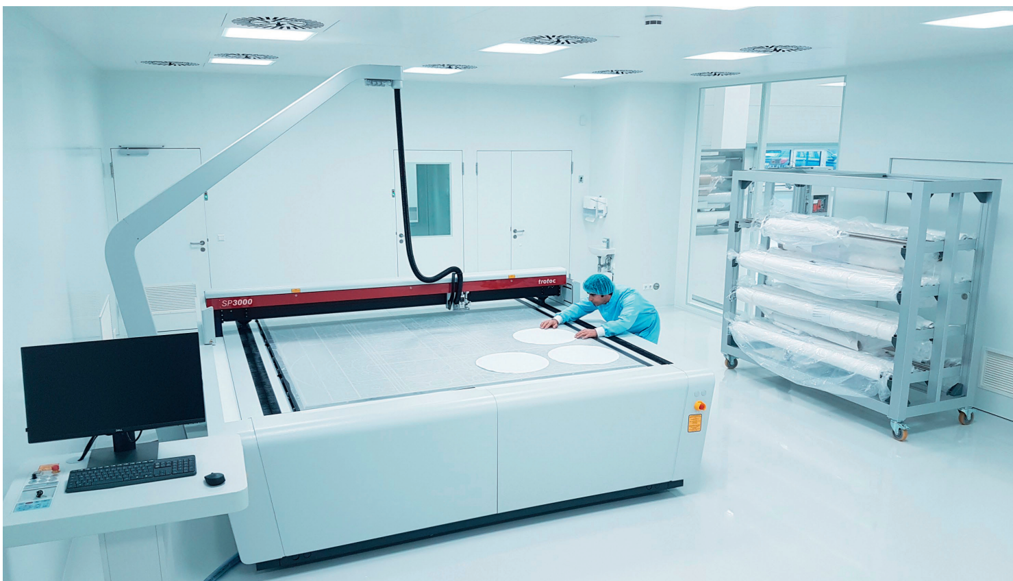
The flatbed laser used in the cleanroom: suction and cooling are installed in the false ceiling outside the cleanroom. © Kögel
