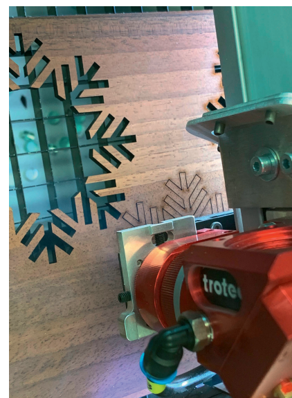
Fig. 2. Precise and contour-sharp cutting is essential for many parts that VIS finishes for their customers. © Visual Information Systems
